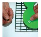
Take the small screw and from the back locate it onto the swivel clip with some washers if needed.
