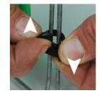
To release the clip press or twist the adjoining parts in opposite directions.
